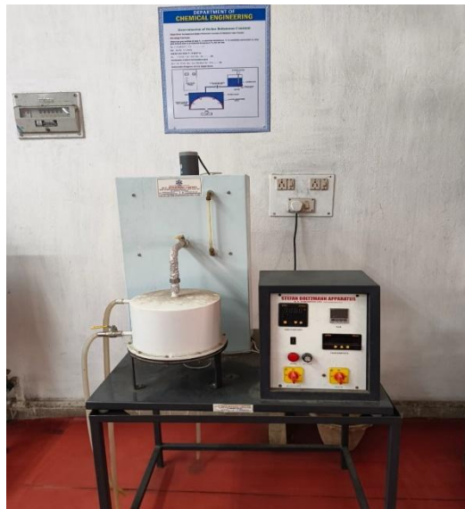
Fig. 7 – Construction of Stefan–Boltzmann Constant experiment
